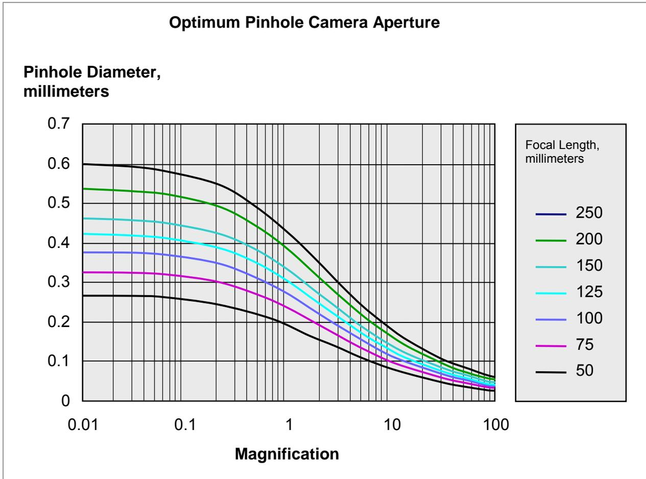
Aperture diameter is rather constant for small magnifications, when the object distance ( $s$ ) is much larger than the image distance ( $f$ ). However, as the object moves closer, the aperture size must be decreased to realize the best focus.
